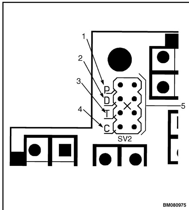
**Figure 15. Jumper Terminal (SV2)**
