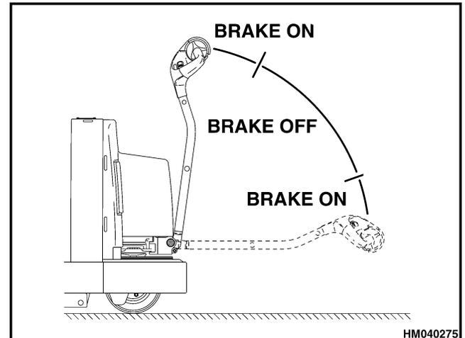
**Figure 11. Brake Operation**
